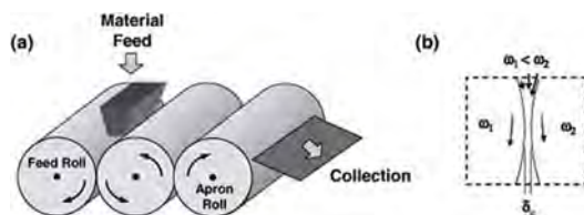
Figure 1. a) Schema of the three roll calendaring, b) high shear zone between rolls. Reprinted with permission from Elsevier. [7]
