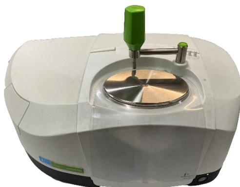
Figure 2.10 FTIR-ATR PerkinElmer spectrometer UATR Two
