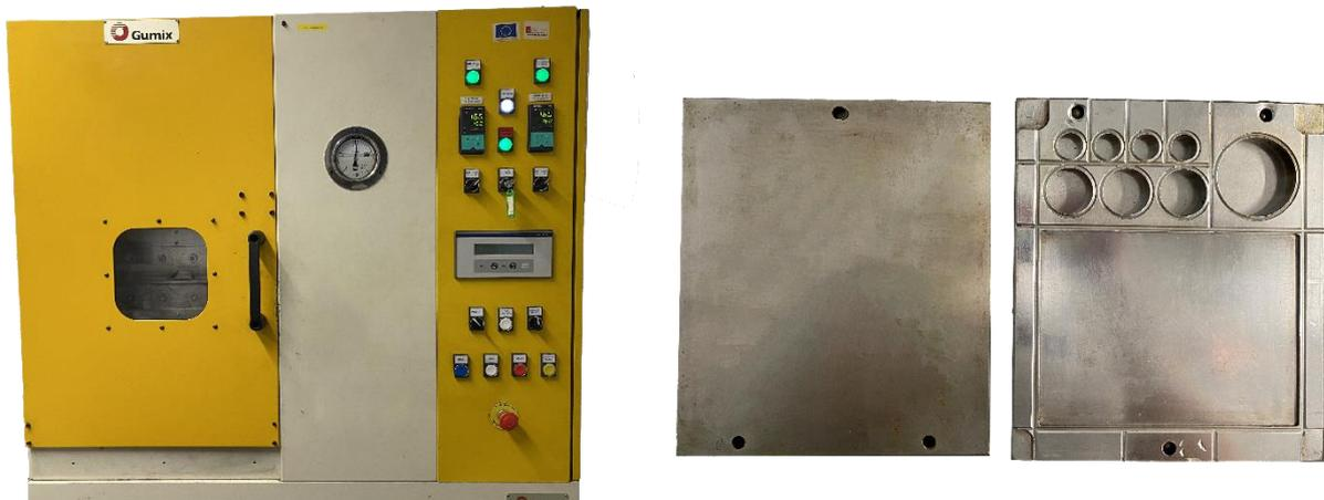
*Figure 2.8 Left: Press (Gumix). Right: Steel molds for different standard test specimens.*
