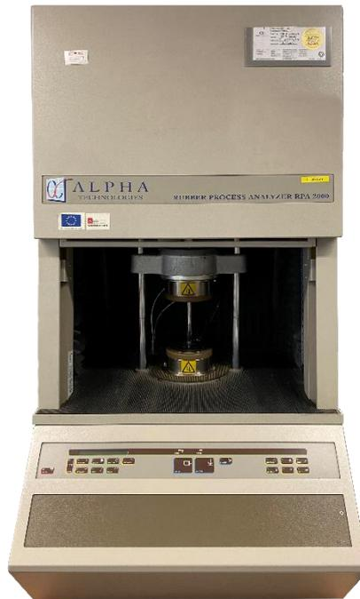
Figure 2.12 Rubber Process Analyzer (RPA 2000, Alpha Technologies).
