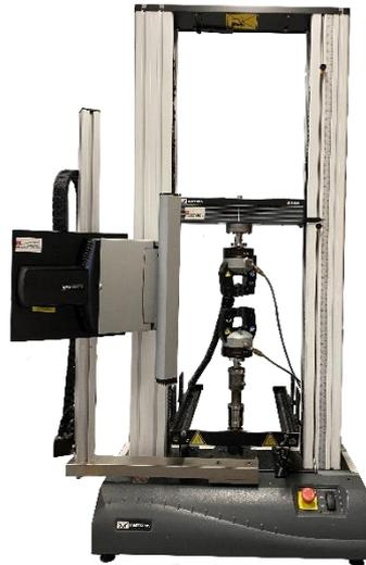
Figure 2.16 Universal mechanical testing machine (Instron 3366).
