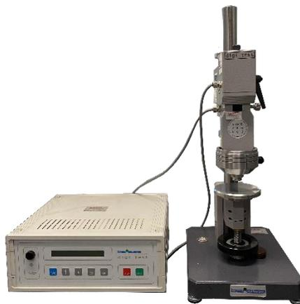
Figure 2.15 Shore A durometer (Bareiss, Neurtek).
